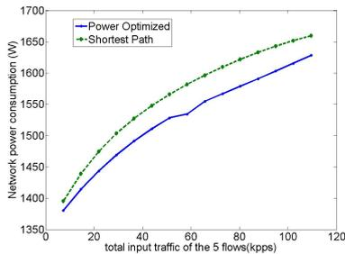
**Figure 1: Power consumption against varying traffic load for power-optimised versus shortest path**
